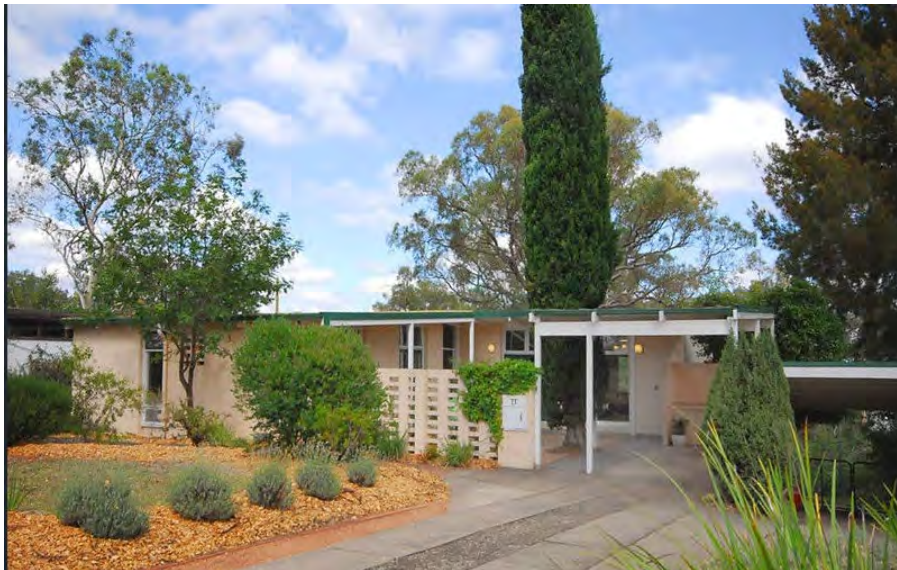
13 Waller Crescent, Campbell, 1962 designed by Theo Bischoff, demonstrates Melbourne Regional style characteristics through the low-pitch gable roof, long, unbroken roofline and narrow edge to roof. (Source: Peter Blackshaw)
