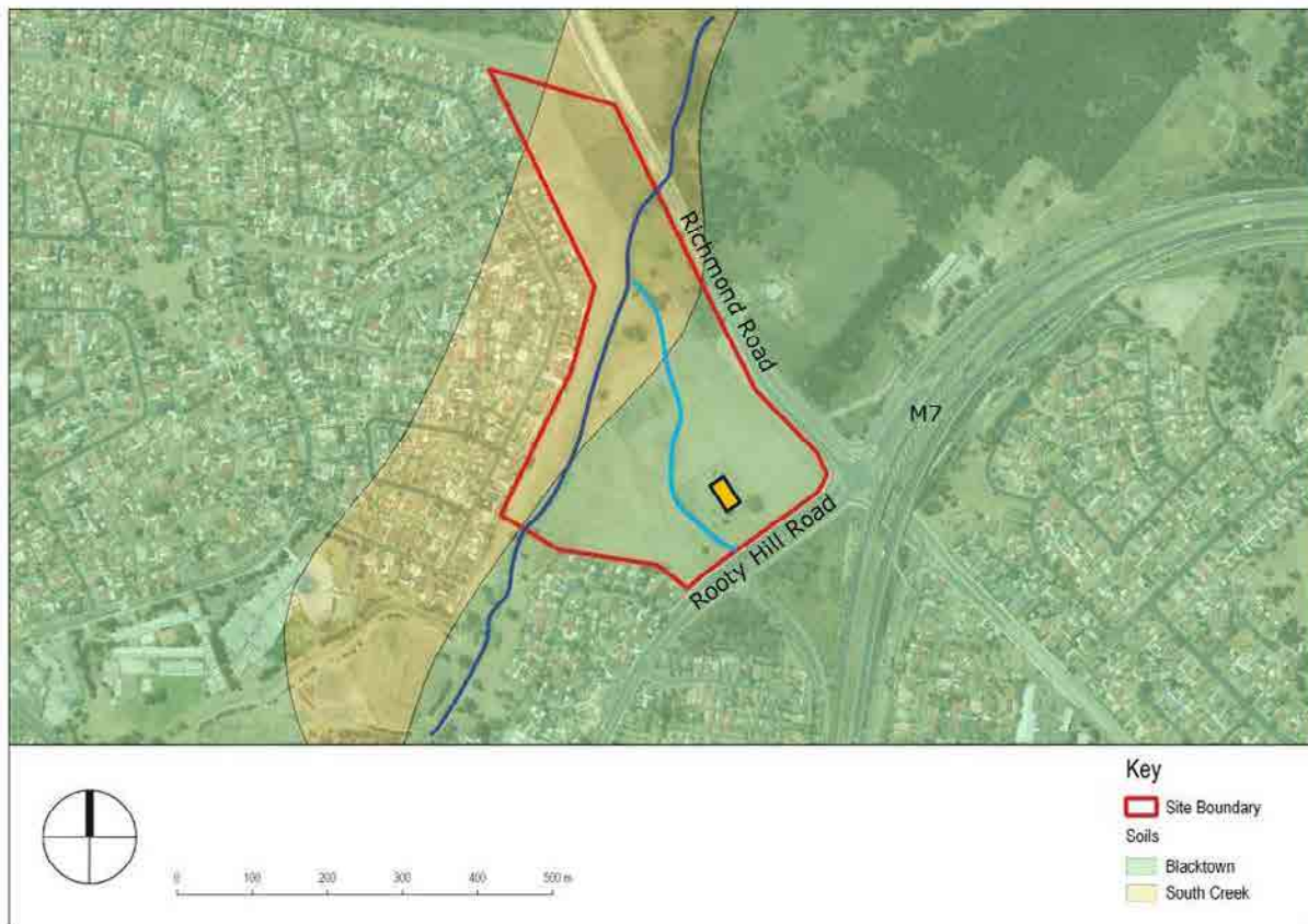
Figure 3.1 Former BNI building (orange), showing the soil landscapes with South Creek alluvium adjacent to Bells Creek (dark blue line). Upslope the soil landscape becomes the residual Blacktown. A recent drainage channel has a course from south to north intersecting with Bells Creek (light blue line). Bells Creek has been significantly altered over the past 70 years. (Source: Google Earth, Department of Lands, with GML additions)
